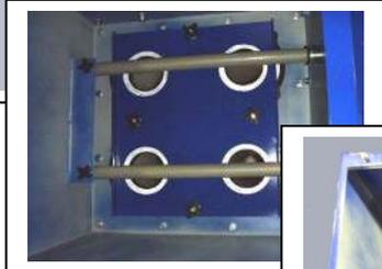
Unscrew knobs securing jet tubes and withdraw jet tubes from socket.
