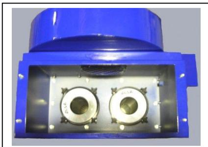
Unscrew and remove the knobs and washers securing the cartridges.
