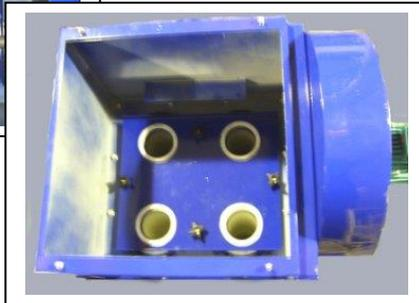
Unscrew and remove the knobs and washers from the cartridge clamping plates. Remove the clamping plates.
