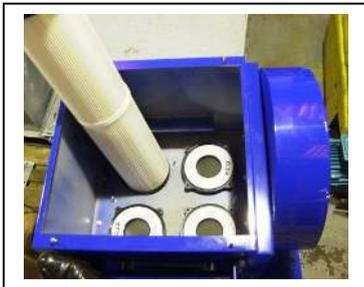
Withdraw the cartridges, shaking them first before extracting to remove excess loose material. **You are strongly advised to replace the black cartridge sealing ring before re-fitting a cartridge.**
