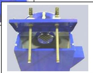
Remove the nuts securing the lid and lift off the lid, putting it in a safe position, so that the wiring and compressed air hose are not stressed.
